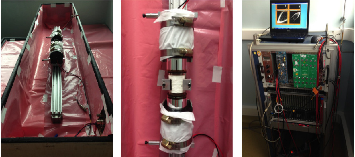
Figure 7.10: Photos of the experimental set-up: the rails on which PMTs are fixed, the cylindrical scintillating plastic surrounded by reflective tape and the electronic rack.
