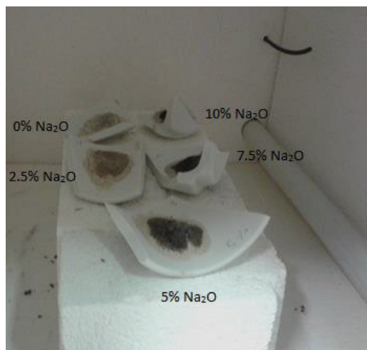
Figure 16 Small scale samples prepared using acetate precursors calcined at 450°C for 5 hours
