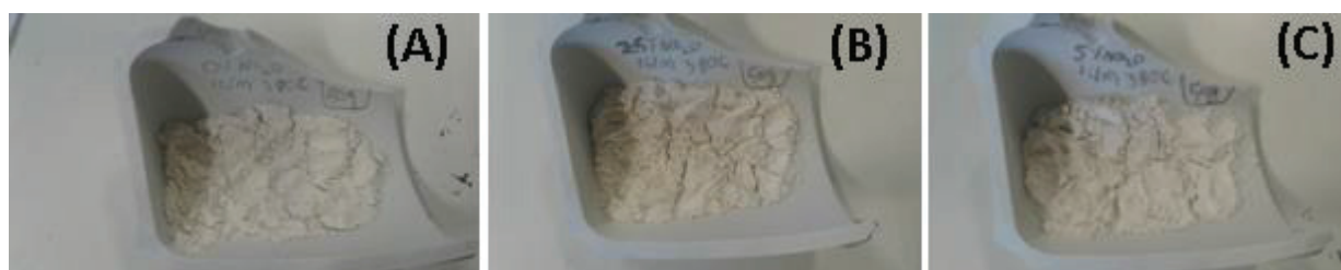
Figure 20 Large scale samples prepared using acetate precursors calcined at 380^{\circ}\text{C} for 5 hours; (A) 10Na MBG (B) 7.5Na MBG (C) 5Na MBG
