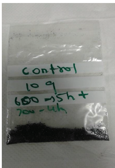
Figure 7 10Na MBG prepared using nitrate precursors after 700°C calcination for 4 hours
