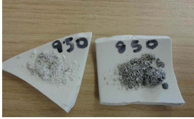
Figure 8 10Na MBG prepared using nitrate precursors after 850°C and 950°C calcination in a gradient kiln
