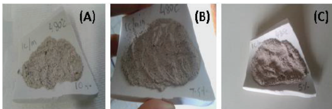
Figure 17 Small scale samples prepared using acetate precursors calcined at 480°C for 5 hours; (A) 10Na MBG (B) 7.5Na MBG (C) 5Na MBG
