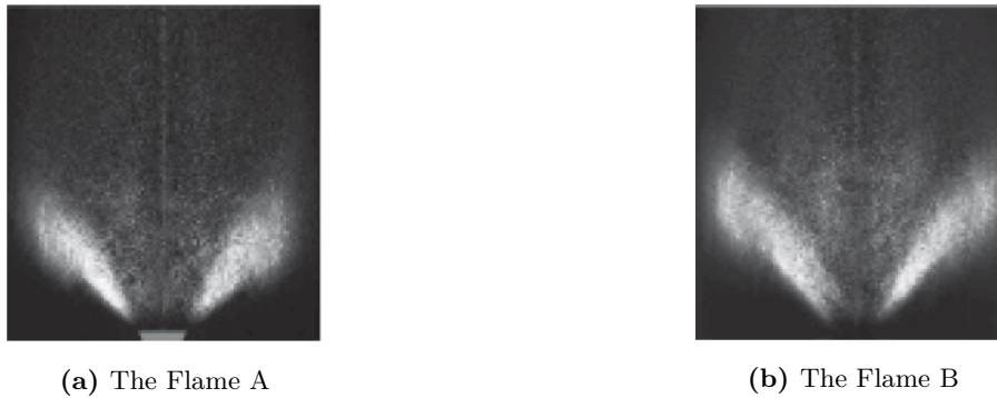
Figure 5.2: Trace of the flame chemiluminescence in the symmetry plane of the burner. From Palies (2010)
