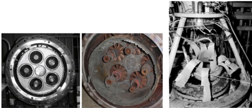
Figure 1.2: Drawbacks of combustion instabilities. Picture (a) shows an injector system damaged after the instability in the combustor (before the instability on the left hand side and after the instability on the right hand side). Picture (b) represents a damaged liquid-rocket engine after combustion instabilities.
