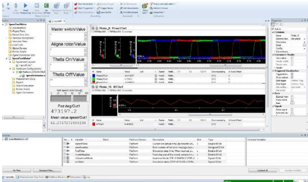
Fig.4.18 ControlDesk interface of the phase current and machine torque for \theta_{on} = 0^\circ and \theta_{off} = 20^\circ
