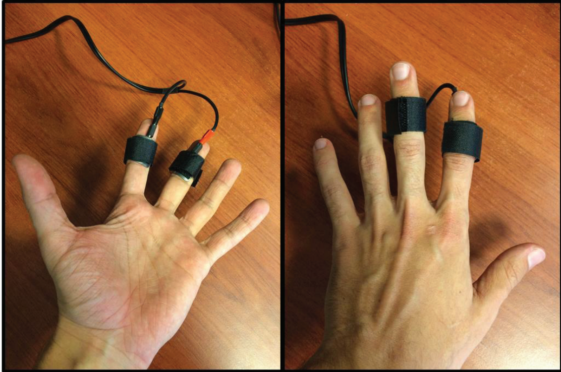
Figure 11. Electrodes positioning for electrodermal activity recordings (MLT116F GSR Finger Electrodes, ADInstruments, Dunedin, New Zeland). Electrodes are always positioned in the index and medium fingers, at the second phalanx (Vernet-Maury et al., 1995).
