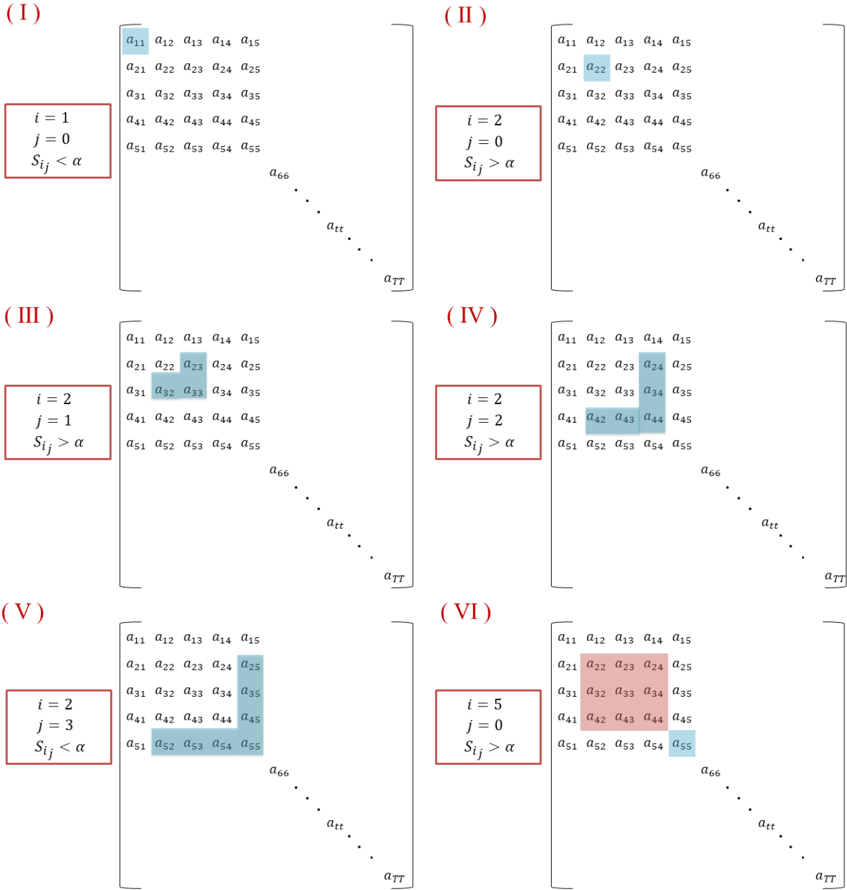
Figure 9. An illustrative example describing the segmentation algorithm
