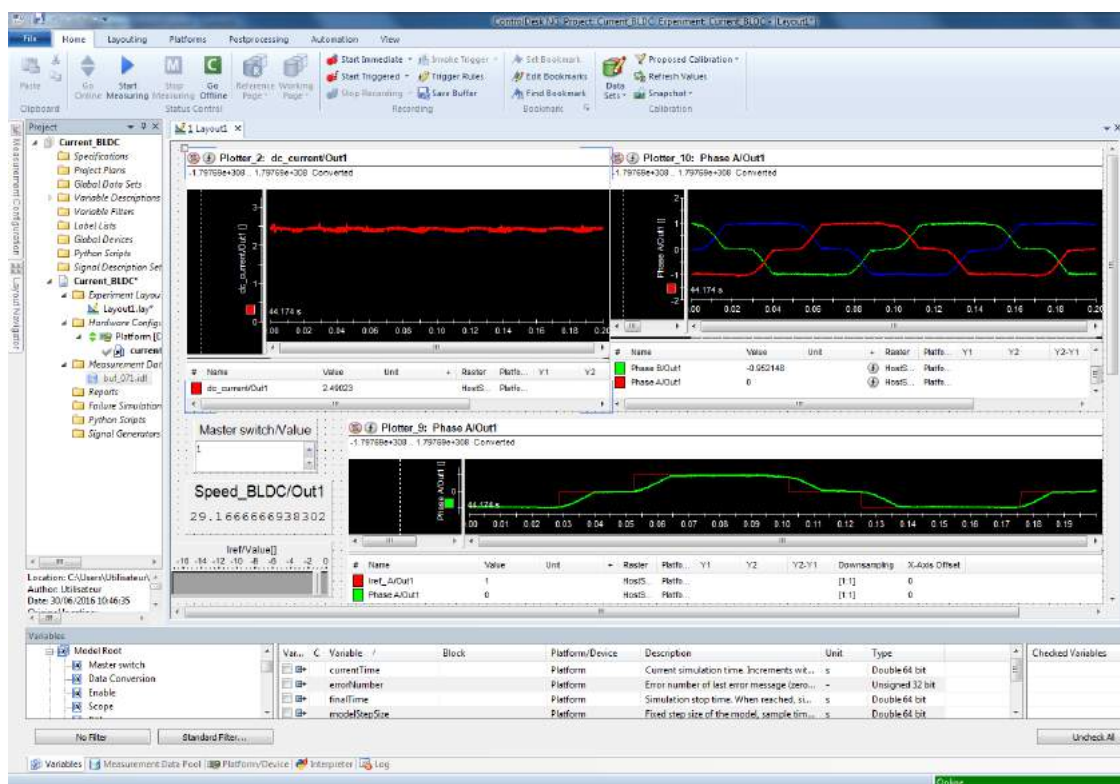
Fig. 5.14. Experimental waveforms of the BLDCPM generator through ControlDesk interface
