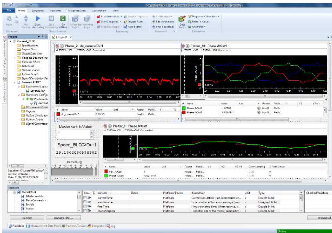
Fig. 5.15. Experimental waveforms of the BLDCPM generator through ControlDesk interface
