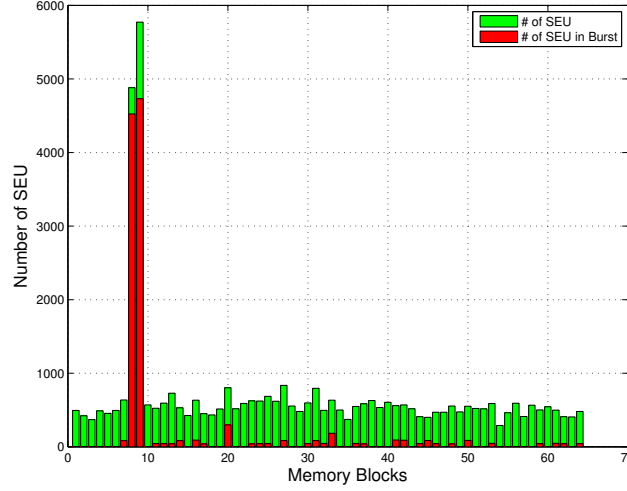
Fig. 3.7: Number of bit upsets per SRAM block, SEU_{block} (green) and SEU_{burst} per SRAM block (red) in one example run. All SEU recorded during irradiation are shown.
