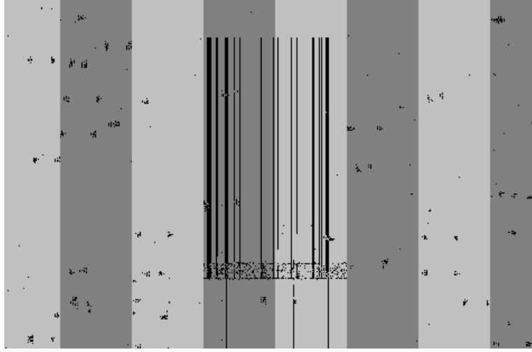
Fig. 3.6: Example of a burst event involving several bit upsets on adjacent rows and error bits located on the same column arrays. Memory blocks are highlighted with different shades of grey.
