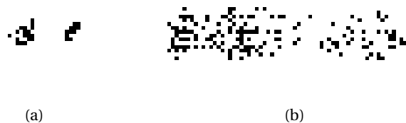
Fig. 3.3: Examples of a small cluster of bit upsets (a) and a burst event characterized by several single bit upsets following a rectangular geometrical shape (b).
