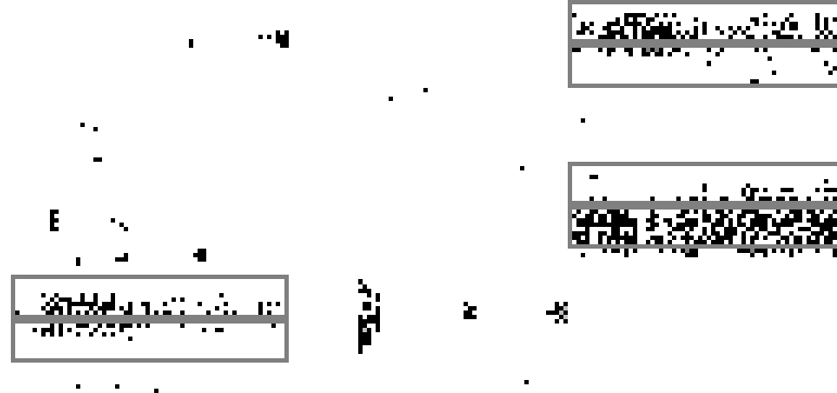
Fig. 3.9: SEU map of the SRAM during irradiation with an alternate blocks algorithm. The rectangles correspond to the detection window at the location where a burst event was recognized.
