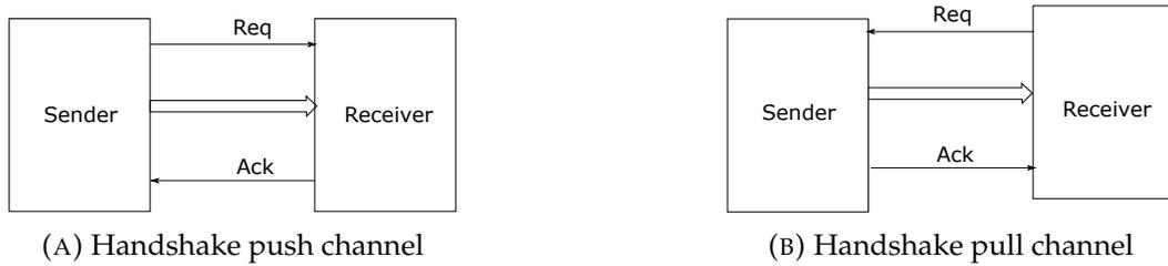
FIGURE 5.11: Handshake push vs. pull channel
