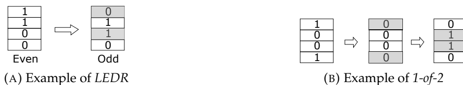
FIGURE 5.20: Transition of two logical bits from (1,0) to (0,1) using LEDR and 1-of-2 protocol. Shaded box represent signal transition
