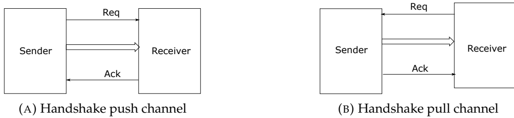
FIGURE 5.11: Handshake push vs. pull channel
