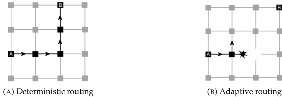
FIGURE 2.2: Deterministic vs. Adaptive routing
