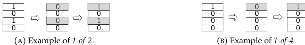
FIGURE 5.18: Transition of two logical bits from (1,1) to (1,1) using dual-rail 1-of-2 and 1-of-4 protocol. Shaded box represent signal transition
