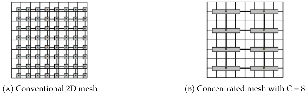
FIGURE 2.13: 64-node on-chip network using (a) 2D mesh and (b) concentrated mesh. C : concentration
