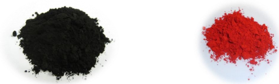
Figure II-2: Cuprous and cupric oxide powders
