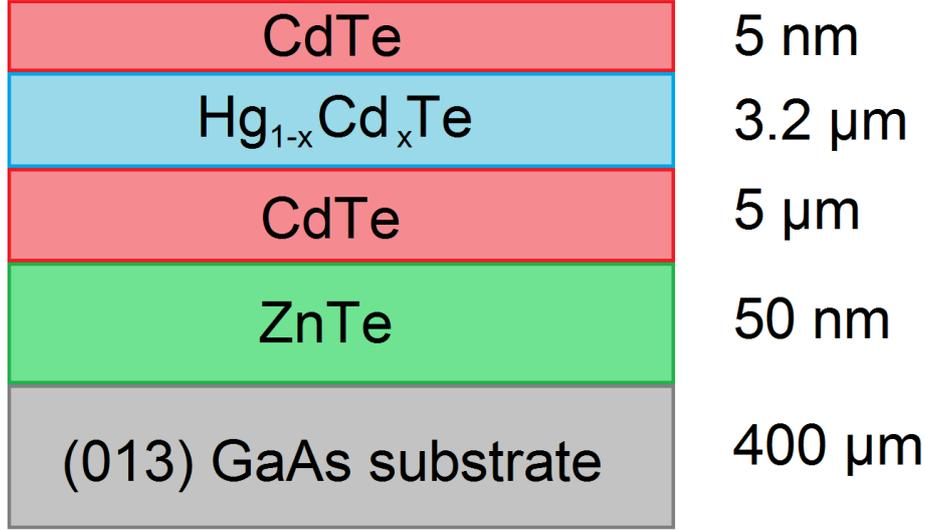
Figure 3.5: Layer structure of  $Hg_{1-x}Cd_xTe$  bulk samples. The cadmium content was equal to  $x_A = 0.175$  and  $x_B = 0.155$  for samples A and B, respectively. The active region of the system is composed of an approximately  $3.2 \mu\text{m}$  thick  $Hg_{1-x}Cd_xTe$  layer, marked on blue on the sketch.
