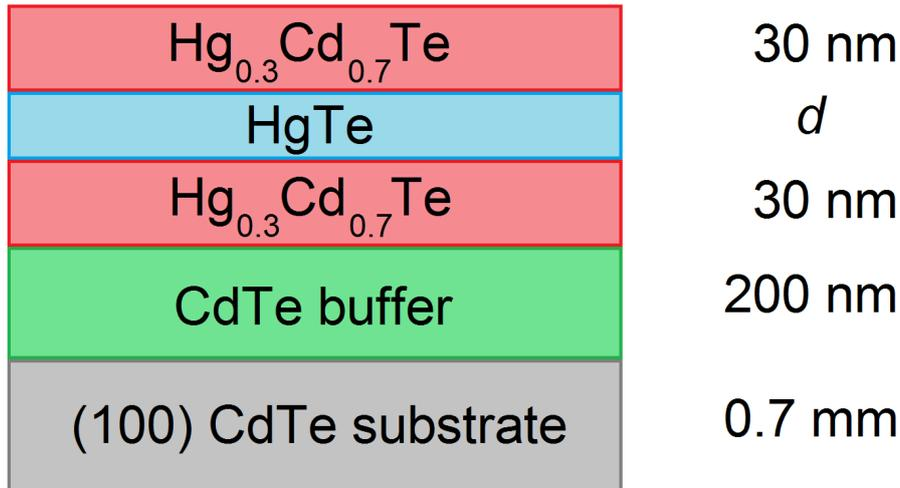
Figure 4.35: Layer structure of investigated films. The active region of the system is composed of a strained HgTe layer with thicknesses  $d = 50$  nm, 25 nm, and 15 nm for Sample A, B, and C, respectively.
