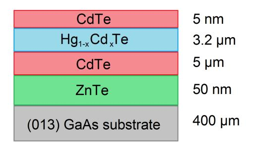
Figure 3.5: Layer structure of  $Hg_{1-x}Cd_x$  Te bulk samples. The cadmium content was equal to  $x_A = 0.175$  and  $x_B = 0.155$  for samples A and B, respectively. The active region of the system is composed of an approximately 3.2 µm thick  $Hg_{1-x}Cd_x$  Te layer, marked on blue on the sketch.
