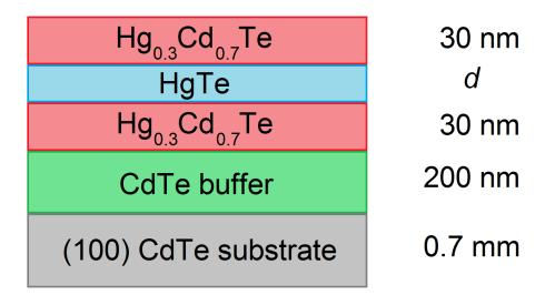
Figure 4.35: Layer structure of investigates films. The active region of the system is composed of a strained HgTe layer with thicknesses d = 50 nm, 25 nm, and 15 nm for Sample A, B, and C, respectively.
