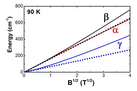
Figure 4.27: Energy evolution of transitions  $\alpha$ ,  $\beta$ , and  $\gamma$  as a function of  $\sqrt{B}$  at T = 90 K approximated by Dirac Hamiltonian (dotted curves) and calculated using 8-band Kane Hamiltonian (solid curves).
