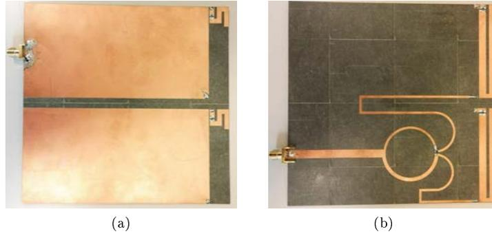
Figure 4.47: Prototype of the array. (a) Top view, (b) bottom view.
