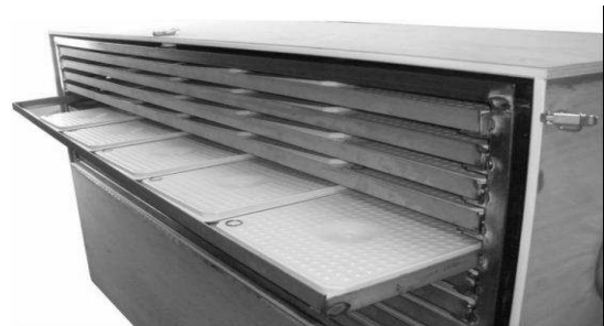
Figure i.17 – LHTES test bench used in the Sumbiosi house.
