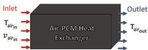
Figure 4.4 – Global domain proposed for the modeling of an air-PCM heat exchanger. The inlet is given by the indoor conditions of the room and the outlet conditions are the air-cooling contribution of the exchanger to the room.
