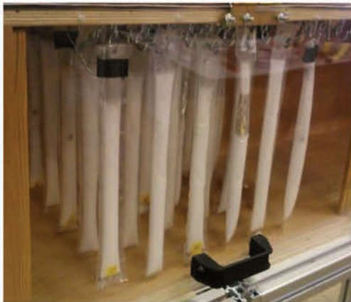
Figure i.20 – Plastic bags used as PCM containers [67].
