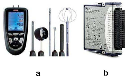
Figure 3.9 – Metrology used on the test bench: a) AMI 300 KIMO® airflow measurement kit [70], and b) National Instruments® NI 9312 data acquisition for temperature measurements [74].
