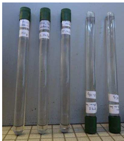
Figure D.2 – Experimental test for tube degradation and leakage using RT21 PCM and water contained inside the PET tubes
