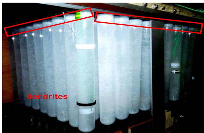
Figure 3.39 – t = 30 min. Once the first half hour of the cycle has passed, we can observe the crystallization starting at the top of the tubes.
