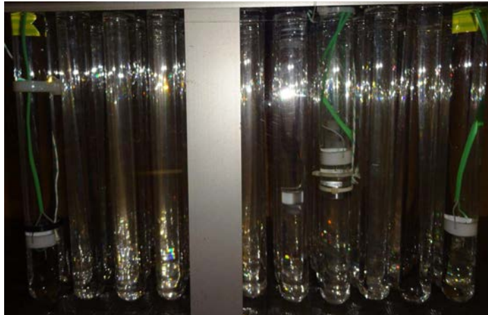
Figure 3.37 – t = 0 . At the beginning all the PCM is in liquid state, following a melting cycle.
