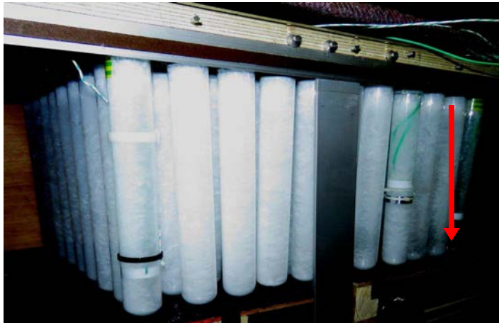
Figure 3.40 – t = 45 min. The crystallization process follows an axial direction along the tube, as can be observed in the last rows of the heat exchanger.
