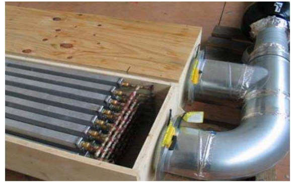
Figure i.15 – The view of an open heat exchanger and a closed heat exchanger connected to an air network.
