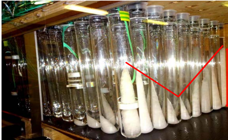
Figure 3.26 – t = 245 min. Almost all the PCM has melted, except for the last rows.
