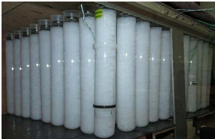
Figure 3.41 – t = t_{final} min. At the end of the cycle all the PCM is fully crystallized.
