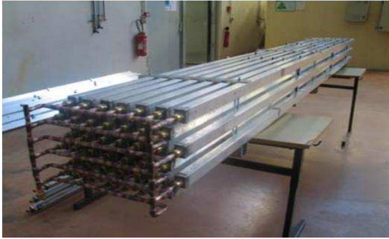
Figure i.14 – One box shape tube bundle containing the PCM.
