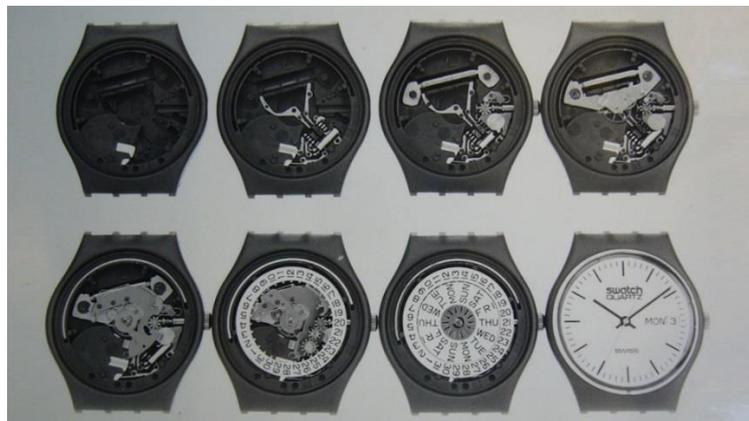
*Figure 21: Assembly of the Swatch<sup>10</sup>*
