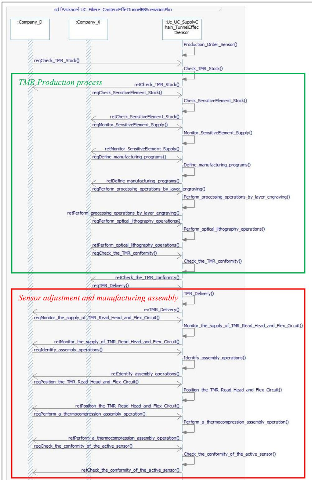
Figure 63: Sequence diagram of the “Sensor production”
