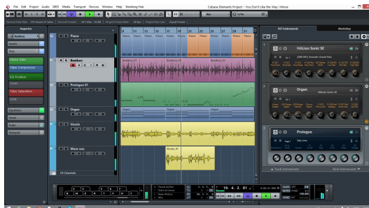
(a) A screenshot of the Cubase audio sequencer. Audio and MIDI tracks are arranged horizontally, with the possibility of having multiple clips on each track.
