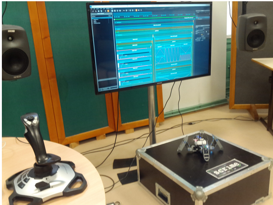
(a) The hardware set-up: a joystick and a Metabot.
