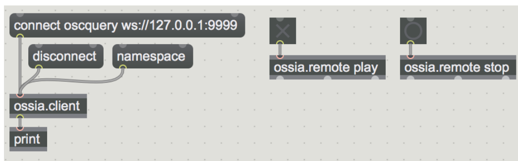
Figure 10.9.: A libossia -based Max/MSP patch to control score . The ossia.client device is used to enumerate the remote device. Two ossia.remote objects allow to control the /play and /stop parameters of score : the first one is a boolean, the second an impulse; the type conversions are handled automatically by the ossia.remote object. Note that there is no need to specify an absolute address: parameters are aware of their hierarchy level and will try to find a corresponding node in the tree according to their hierarchical position in the patches.
