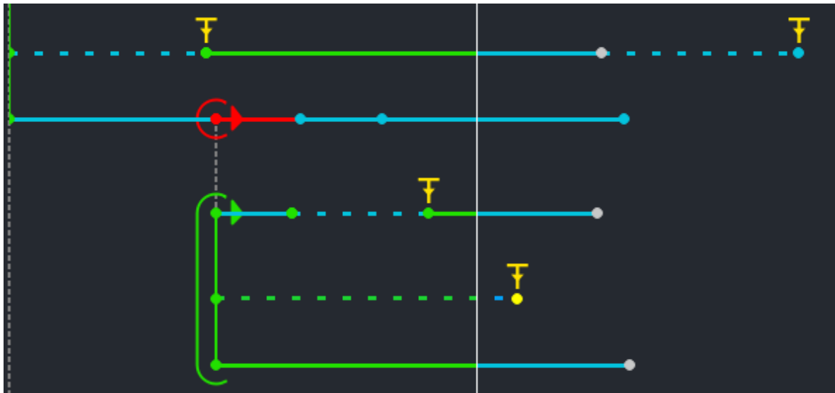
Figure 8.12.: Execution offset. The white bar indicates the point at which execution was requested. Branches with false conditions are discarded, and all other branches are set up as if their run duration had been exactly the nominal duration of the intervals.
