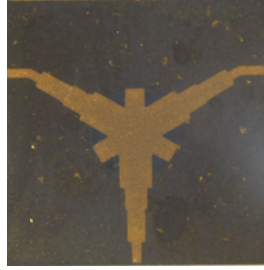
FIGURE 5-21 – Assemblage Y_{1,497}Cu_{0,05}Bi_{0,67}Gd_{0,8}Fe_{4,2}Al_{0,8}O_{12} + V_2O_5 - Y_{2,197}Cu_{0,05}Ca_{0,1}Bi_{0,67}Fe_{4,95}V_{0,05}O_{12} - Or ESL / Design Cobham
