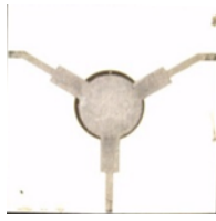
FIGURE 5-6 – Assemblage VLF220 - Y_{2,297}Cu_{0,05}Bi_{0,67}Fe_5O_{12} - Argent ESL / Design Lab-Sticc
