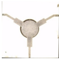
FIGURE 5-6 – Assemblage VLF220 - Y_{2,297}Cu_{0,05}Bi_{0,67}Fe_5O_{12} - Argent ESL / Design Lab-Sticc
