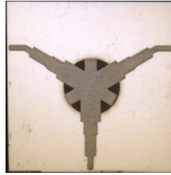
FIGURE 5-4 – Assemblage VLF220 - Y_{2,297}Cu_{0,05}Bi_{0,67}Fe_5O_{12} - Argent ESL / Design Cobham
