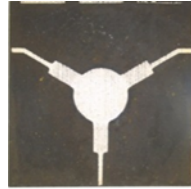
FIGURE 5-19 – Assemblage Y_{1,497}Cu_{0,05}Bi_{0,67}Gd_{0,8}Fe_{4,2}Al_{0,8}O_{12} + V_2O_5 - Y_{2,197}Cu_{0,05}Ca_{0,1}Bi_{0,67}Fe_{4,95}V_{0,05}O_{12} - Argent ESL / Design Lab-Sticc
