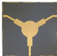
FIGURE 5-23 – Assemblage Y_{1,497}Cu_{0,05}Bi_{0,67}Gd_{0,8}Fe_{4,2}Al_{0,8}O_{12} + V_2O_5 - Y_{2,197}Cu_{0,05}Ca_{0,1}Bi_{0,67}Fe_{4,95}V_{0,05}O_{12} - Or ESL / Design Lab-Sticc
