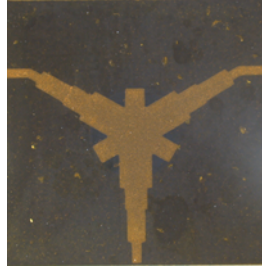
FIGURE 5-21 – Assemblage Y_{1,497}Cu_{0,05}Bi_{0,67}Gd_{0,8}Fe_{4,2}Al_{0,8}O_{12} + V_2O_5 - Y_{2,197}Cu_{0,05}Ca_{0,1}Bi_{0,67}Fe_{4,95}V_{0,05}O_{12} - Or ESL / Design Cobham
