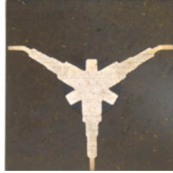
FIGURE 5-17 – Assemblage Y_{1,497}Cu_{0,05}Bi_{0,67}Gd_{0,8}Fe_{4,2}Al_{0,8}O_{12} + V_2O_5 - Y_{2,197}Cu_{0,05}Ca_{0,1}Bi_{0,67}Fe_{4,95}V_{0,05}O_{12} - Argent ESL / Design Cobham
