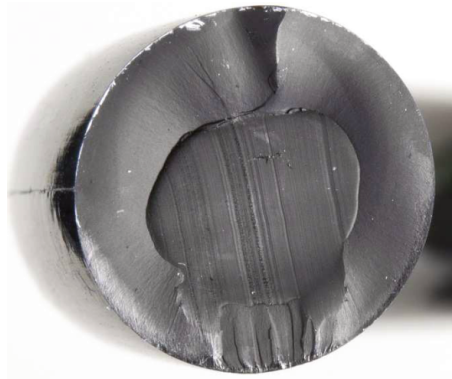
Figure 5.1-5 – Photo of a cut cross-section of HNBR aged for 101 days at 150°C in uncompressed state (Kömmling et al. 2016).
