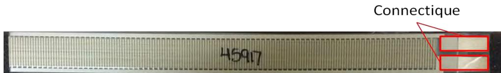
**Figure 166: PFC-W14 (AFC) (Advanced Cerametrics Inc.)**
