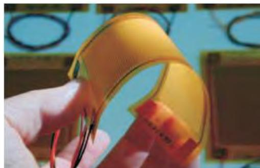
Figure 84: Capteur MFC (Source: [www.smart-material.com](http://www.smart-material.com))
