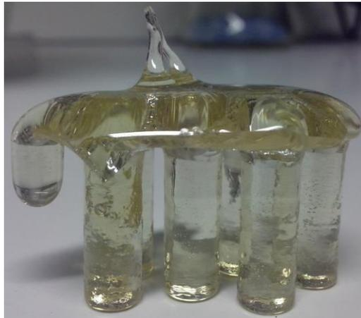
Figure II.5. An example of glass produced by pouring melt into a graphite mould.
