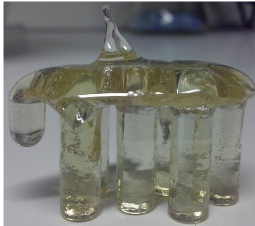
Figure II.5. An example of glass produced by pouring melt into a graphite mould.
