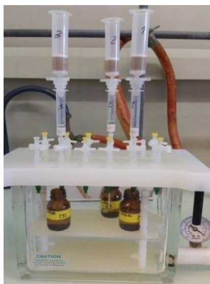
Figure III.8: Coupling between the MSPD cartridge containing the sediment and the MIP-phenolic, to selectively sorb OH-PAHs.
