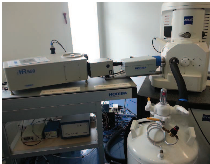
Figure II.16. Picture of the CL spectrometer available at LSPM. In the bottom of this image it is possible to see a bottle of liquid nitrogen which allowed of investigated the sample at the temperature of 110 K.
