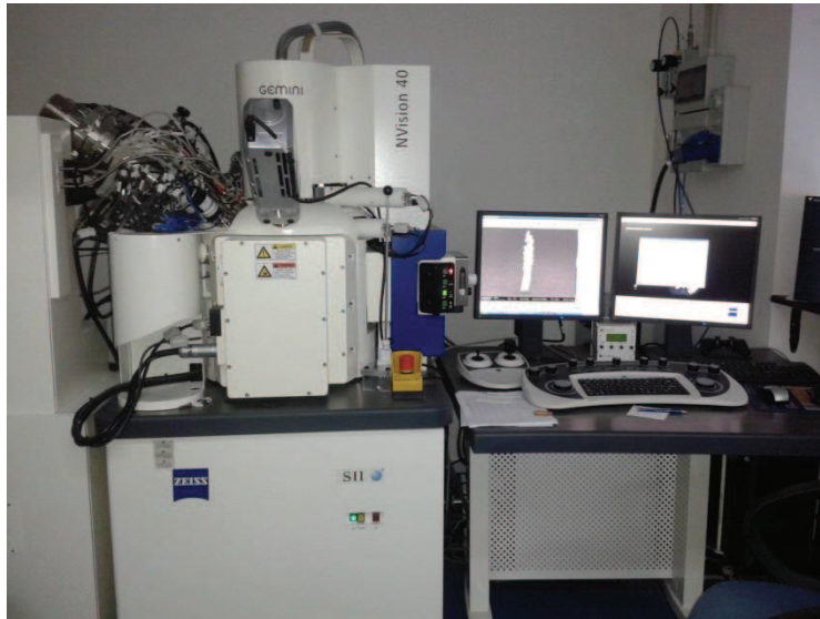
Figure II.13. Picture of the SEM microscope at the CNR-IMM Institute for Microelectronics and Microsystem of Lecce (Italy).
