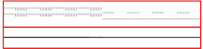
Fig. 5. Zoomed-in example of a single type C cluster, as it appears on physical (top) and logical (bottom) bitmaps.
