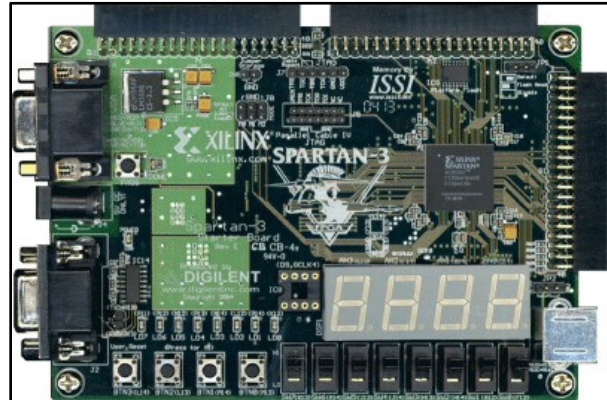
Figure 32: Top view of the Digilent Spartan-3 Starter Board (DSSB).
