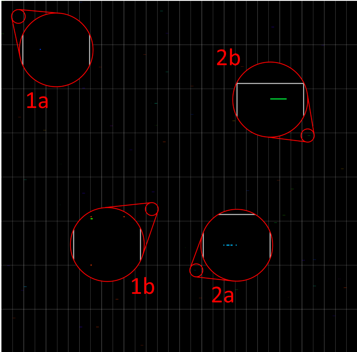
Figure 66: Logical bitmap from an anti-Gray dynamic stress test with krypton ( LET\ 32\ MeV.cm^2.mg^{-1} ).
