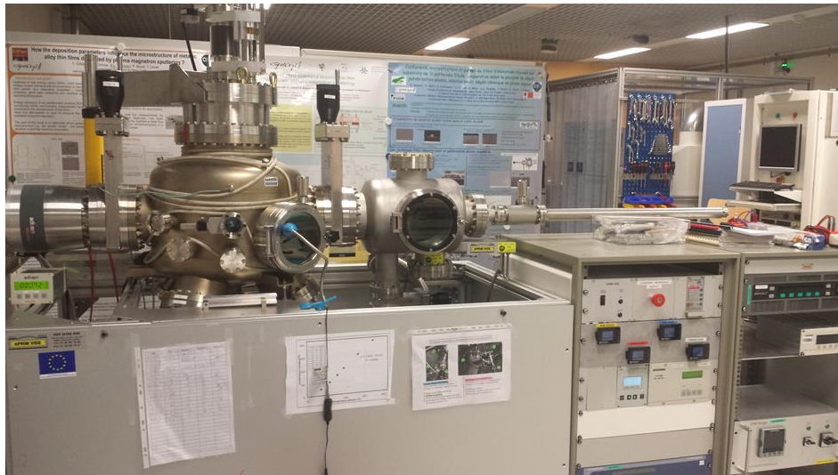
Figure.V.1. Photo of experimental setup used for magnetron sputtering deposition of titanium oxide thin film.
