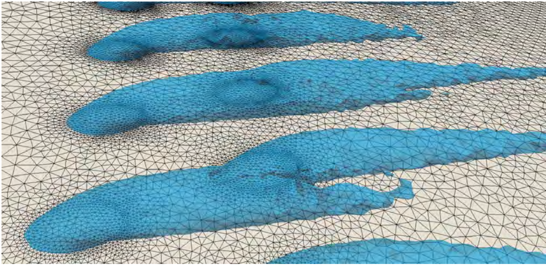
Figure 5.8: Isosurface of the coolant jet allowing to visualize the boundary mesh in the modeled case. Extrated from [80]
