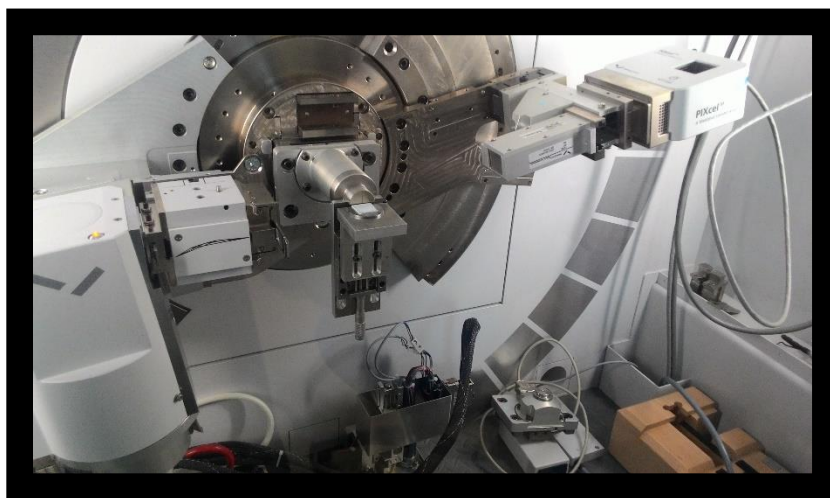
Fig. 72. PANalytical diffractometer with a design of low incidence X-ray.
