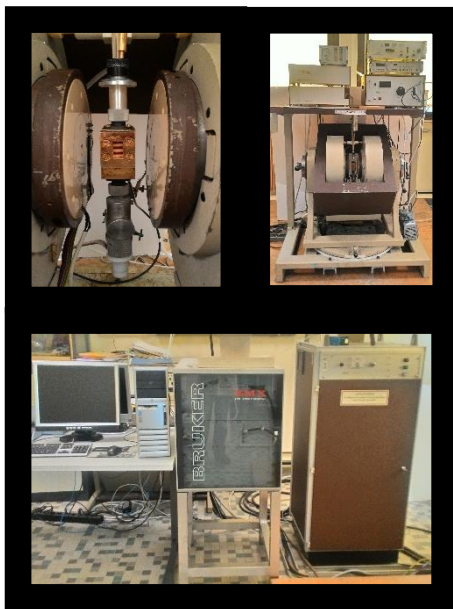
Fig. 77. EPR equipment, Bruker EMX.
