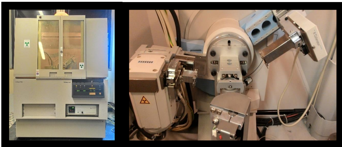
Fig. 71. PANalytical \theta/\theta Bragg- Brentano X'pert MDP PRO diffractometer for measurements of powders.
