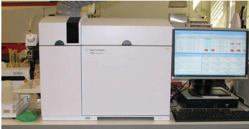
**Figure II.15.** ICP-MS type Agilent 7700X
