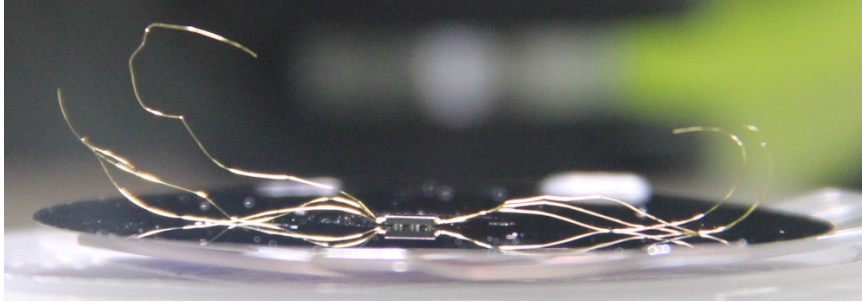
FIGURE 6.9: The light detector with the coupled NTD sensor. Between the two surfaces one can see the array of separated glue spots.
