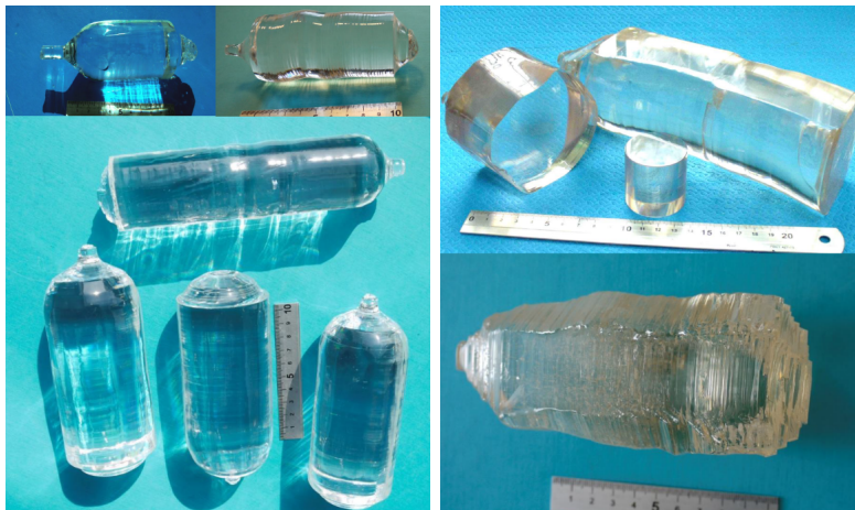
FIGURE 4.2: The Li_2MoO_4 crystal boules (left), and ZnMoO_4 crystal boules (right). ZnMoO_4 boules have less homogeneous structure due to difficulties in crystal growth.
