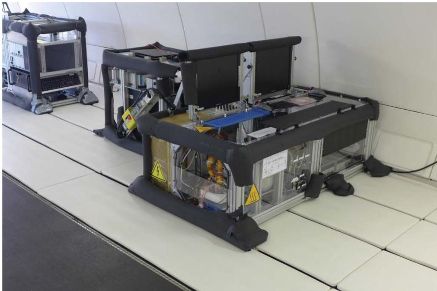
Figure III.23: Experimental facility installed and ready to operate in the plane.
