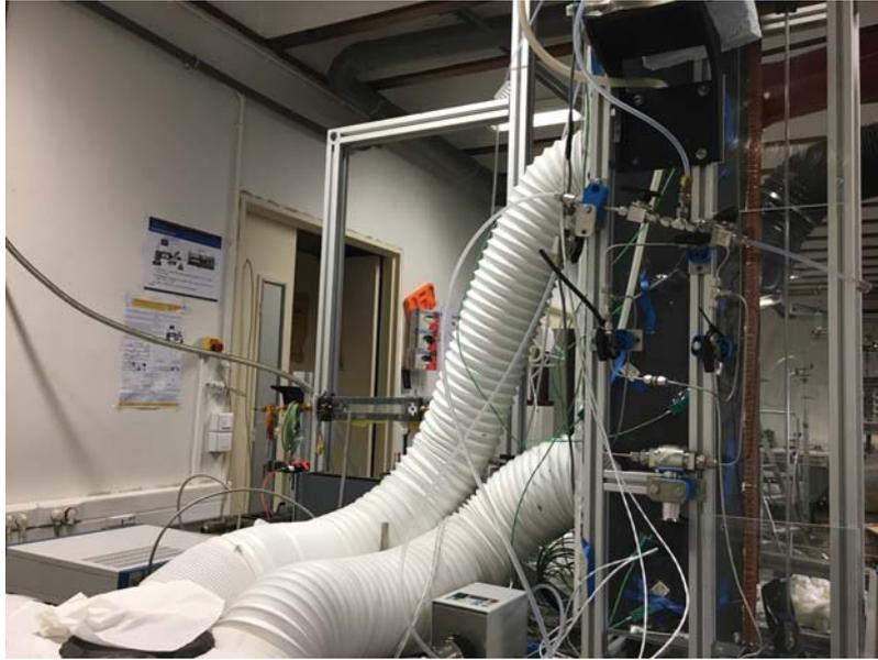
Figure IV.3: The air-conditionner conduct for the secondary fluid
