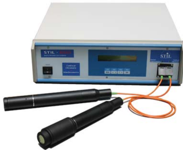
Figure IV.5: The complete STIL DUO employed to measure liquid film thickness with two pencils: one for confocal mode and one for interferometer mode.
