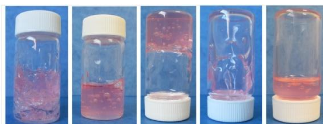
Figure 5.13. Gel formation by mixing PMMA BE 3 and X 1 and subsequent creep at room temperature. First image: gel broken with a spatula. 2 nd and 3 rd images: after 48 hours, 4 th image: 96 hours, 5 th image: 192 hours.
