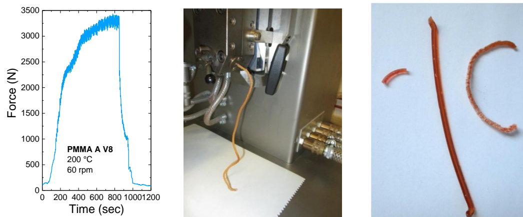
Figure 3.7. From left to right: Raw data from extrusion of PMMA A V8 . Picture of the vitrimer PMMA A V8 during and after extrusion.
