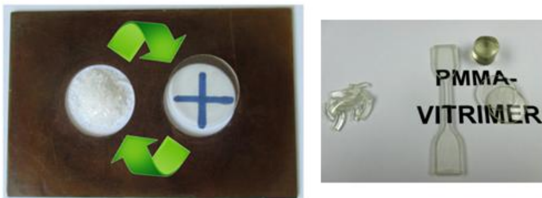
Figure 5.14. Processing and reprocessing of PMMA BE V3 by compression molding. The colorless powder was compression molded at 150 °C for 30 minutes under a load of 3-5 tons.
