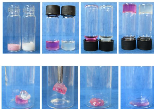
Figure 5.12. Top row: gel formation of pink (left vial) and discolored (right) PMMA BE 3 in dried THF. Bottom row: Sticking of gels at room temperature, from left to right: after contact, after 2 hours, 5 hours and 24 hours.
