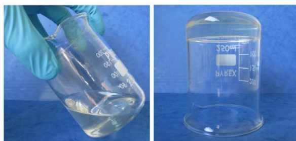
Figure 5.6. Crosslinking of PMMA BE 3 at room temperature in solution. Left side: Solution of the functional thermoplastic in dried THF (25 wt%). Right side: The resulting vitrimer gel right after gel-formation, ca. 10 min after the addition of the bisboronic ester crosslinker \mathbf{X}_1 .
