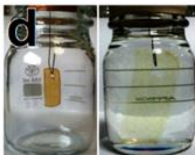
Figure 3.11. Top: Swelling characteristics of PBMA A V1 at room temperature. Bottom: Solubility tests on a processed (compression molding, 150 °C, 1 h) sample PBMA A V1 (650 mg, 100 mL anisole). Left side: before heating, right side: after heating to 120 °C in anisole overnight.
