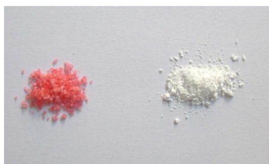
Figure 5.2. Functional PMMA copolymers P3a and P3b . Pink powder = PMMA polydiol with a dithioester chain-end (corresponding to the RAFT CTA), P3a . White powder = PMMA poly(boronic ester) with no dithioester chain-end, P3b .
