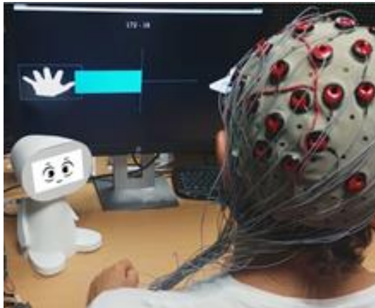
Figure 4. Brain Computer Interface training during which PEANUT (on the left) provides user with social presence and emotional support adapted to his performance and progression [64].
