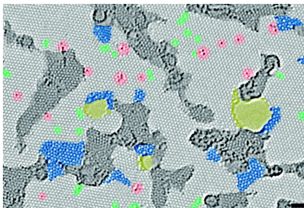
Figure 3.14: RGO obtained by hydrogen plasma treatment. Contaminated regions are shaded in dark gray, desordered regions in blue, individual ad-atoms or substitutions in red, isolated defects in green and holes in yellow. The scale bar is 1 nm [26].
