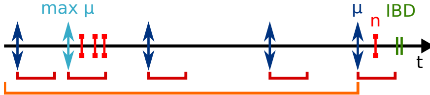
Figure 9.1 – Selection of the \mu yielding the maximum posterior probability that the prompt from the IBD candidate (green) is a cosmogenic decay. The n = 3 neutrons (red) generated by the maximal \mu (light blue), certainly help maximising P(co | n, d) . Note that \mu 's closer in time do not have more chances to be selected. Due to the after- \mu veto (red), \mathcal{W}_p (orange) must be offset.
