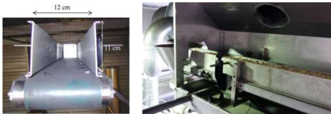
Figure 45. The conveyor belt (used in continuous operation mode): front view (left) and side view (right)
