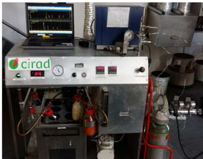
Figure 47. Photo of the sampling system for condensable and gas
