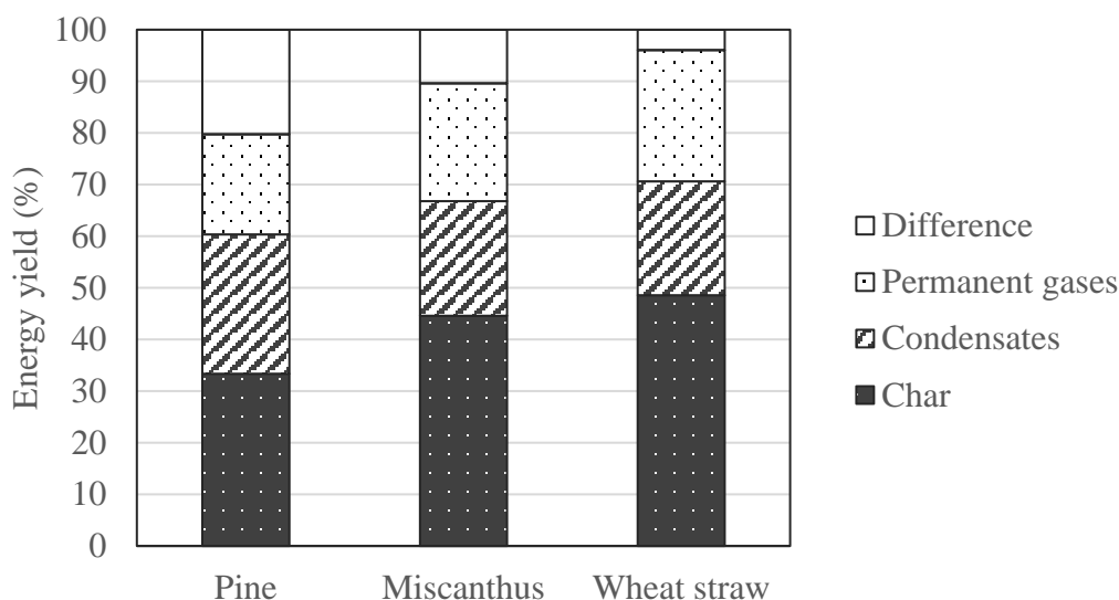
Figure 61. Energy yields of the oxidative pyrolysis products from different biomasses, continuous mode and 0.022 \text{ kg}\cdot\text{m}^{-2}\cdot\text{s}^{-1} air flux
