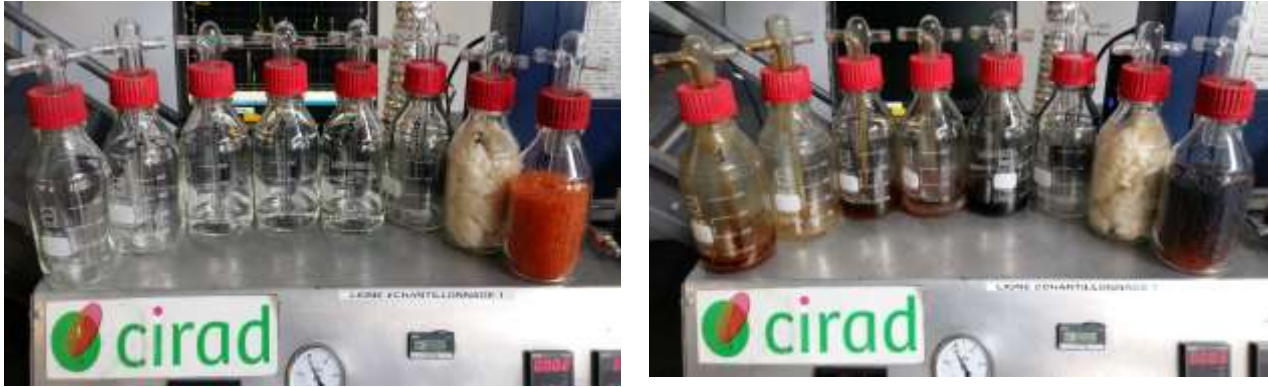
Figure 48. The impingers before (left) and after (right) a test with Pine pellets in continuous mode.
