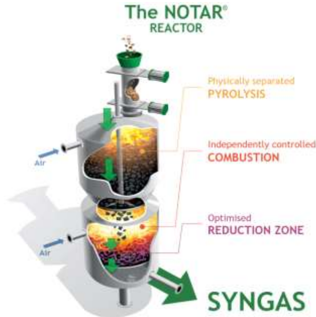
Figure 16. The staged fixed bed gasifier NOTAR ® developed by Xylowatt ®
