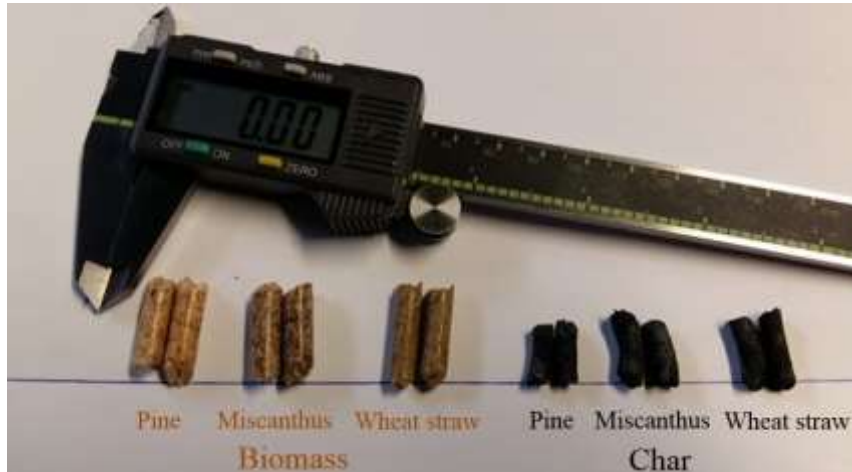
Figure 77. Measurement of particle size of the biomasses and the produced chars
