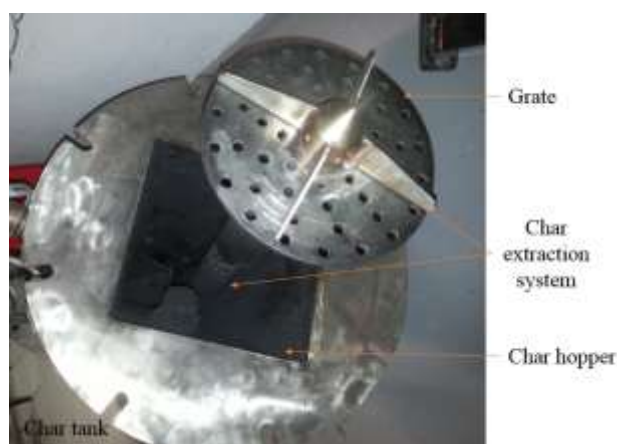
Figure 44. Grate and char extraction system
