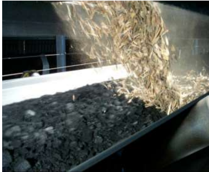
Figure 13. Wood pellets are metered directly on a coal conveyor before the mills at Wallerawang Power Station, Australia [27]
