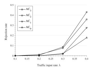
Figure 2.5: Rejection rate for messages of different access classes
