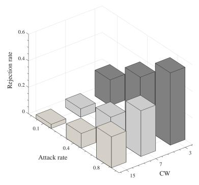
Figure 4.8: Rejection rate as a function of CW size and the attack rate
