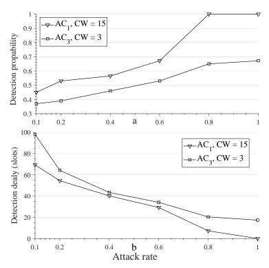
Figure 4.7: Detection probability (a) and delay (b) as a function of the attack rate
