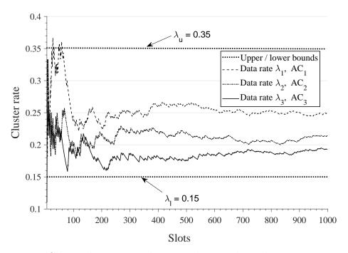
Figure 4.3: Cluster data rate under normal network conditions; no jamming
