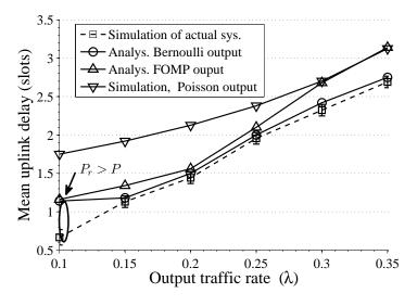
Figure 3.7: Mean uplink delay as a function of the output rate, M=3
