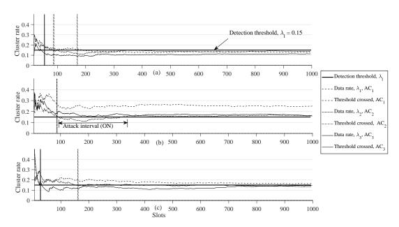
Figure 4.6: The algorithmic performance under different attacker models (a) Constant jammer (b) Random jammer (c) Intelligent jammer
