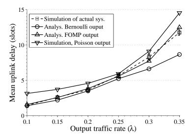
Figure 3.8: Mean uplink delay as a function of the output rate, M=5
