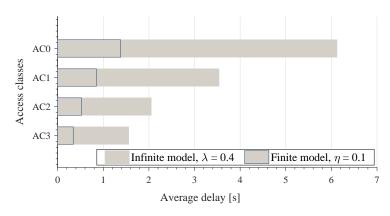
Figure 2.3: Average delay of Finite and Infinite model for different access classes
