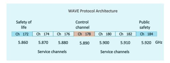
Figure 2.1: DSRC allocated spectrum
