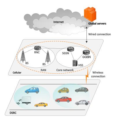
Figure 3.2: DSRC-cellular hybrid architecture
