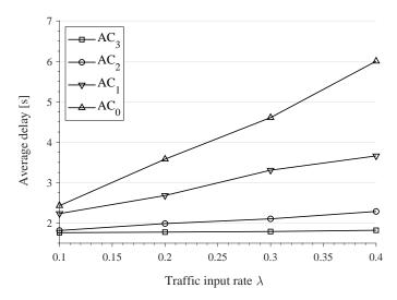
Figure 2.4: Average delay for messages of different access classes
