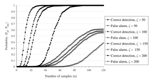
Figure 4.4: Power and false alarm curves for different threshold values
