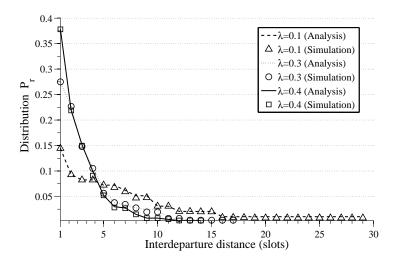
Figure 3.3: Interdeparture distribution for different input traffic rates
