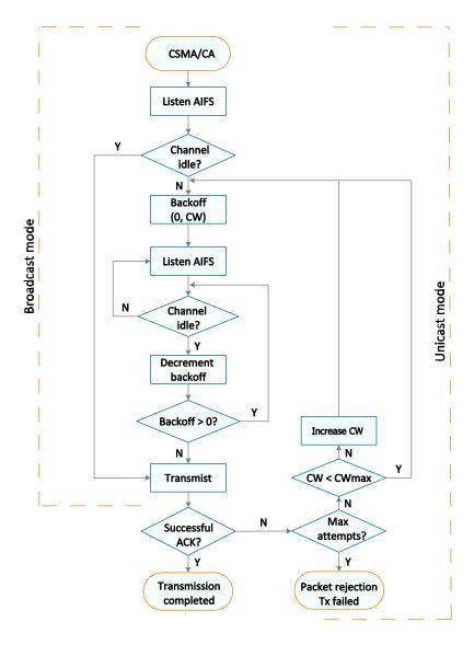
Figure 4.1: CSMA/CA procedure in IEEE 802.11p
