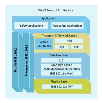
Figure 1.2: WAVE protocol architecture
