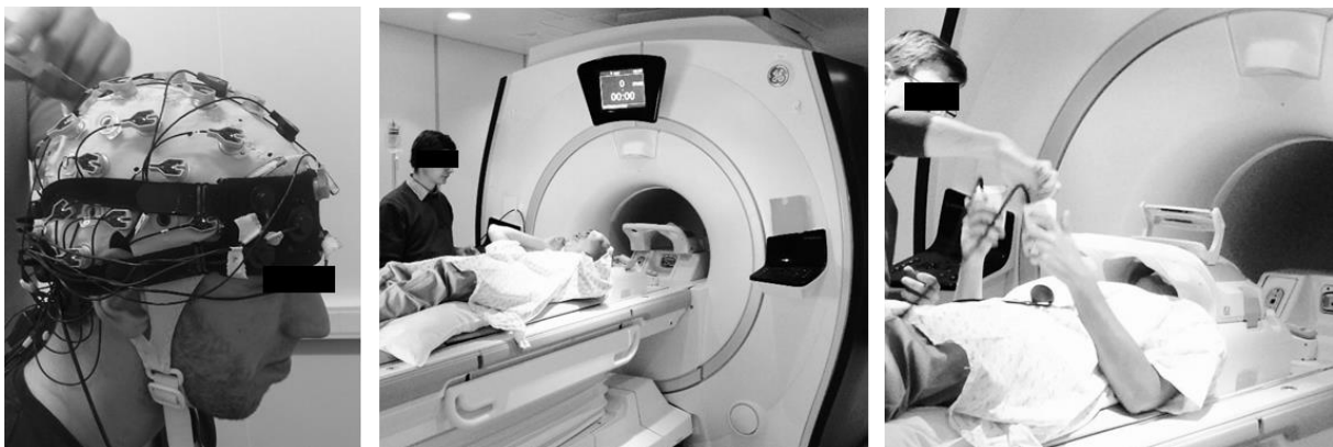
Figure 8. Methods to study the brain. Left: Set-up to measure brain activity by EEG, concomitant with hemodynamic changes in the prefrontal cortex by fNIRS. Middle and right: Functional Magnetic Resonance Imaging (fMRI). Subjects enter the fMRI scanner in supine position, with their head “fixed” and are requested to lay still during the test. Subjects hold a button in each hand which they need to press in response to the stimuli during the cognitive test.
