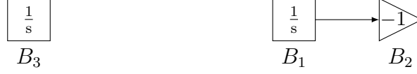
(a): Backward graph of B_3 , input of B_1 (b): Backward graph of B_2 , input of B_3
