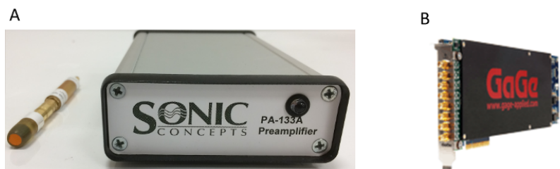
Figure 2.7: Passive cavitation detection A) shows on the left the wide-band frequency hydrophone and the pre-amplifier on the right. B) The acquisition of the signal was performed using a GaGe Oscar (Oscar, 12-bit, 100 MHz sampling frequency, Gage Applied Technologies, DynamicSignal LLC, IL, USA) which can acquire up to 4 channels at 100 MHz.
