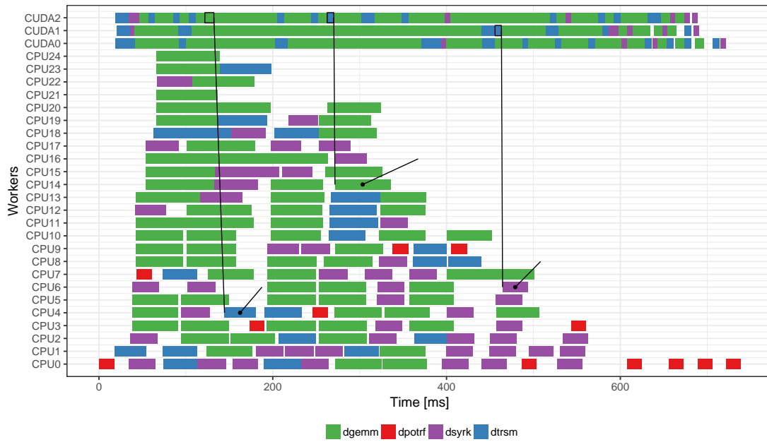
Figure 5.11: Space-time view showing only the last dependency of a some given tasks.
