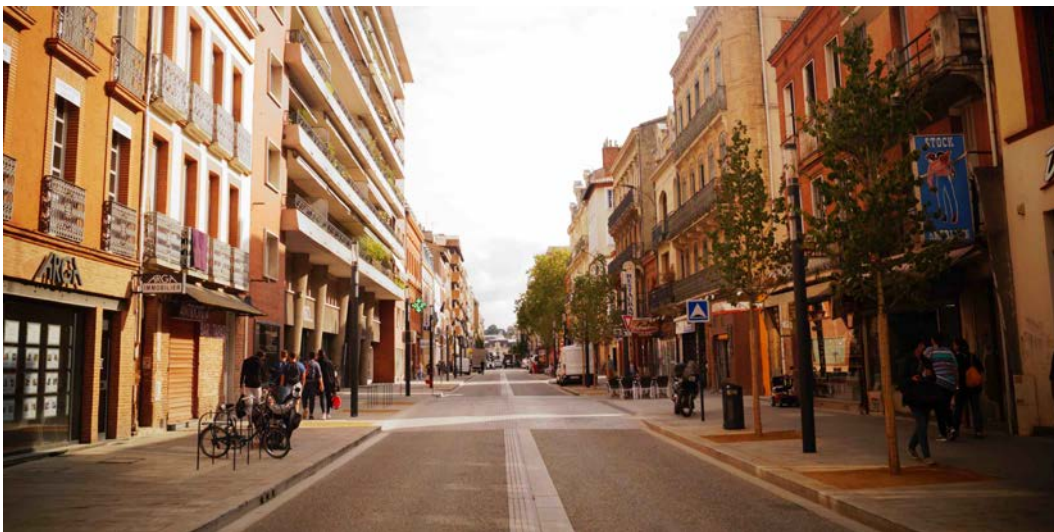
Figure 12 Transformation of the Rue Bayard in Toulouse, France. Rue Bayard had typical city- street profile, but was largely dominated by cars. In the recent refurbishment, sidewalks were enlarged, parking spaces removed, street lights changed, and trees planted ( www.archives.toulouse.fr , www.toulouse-m2ct.com )
