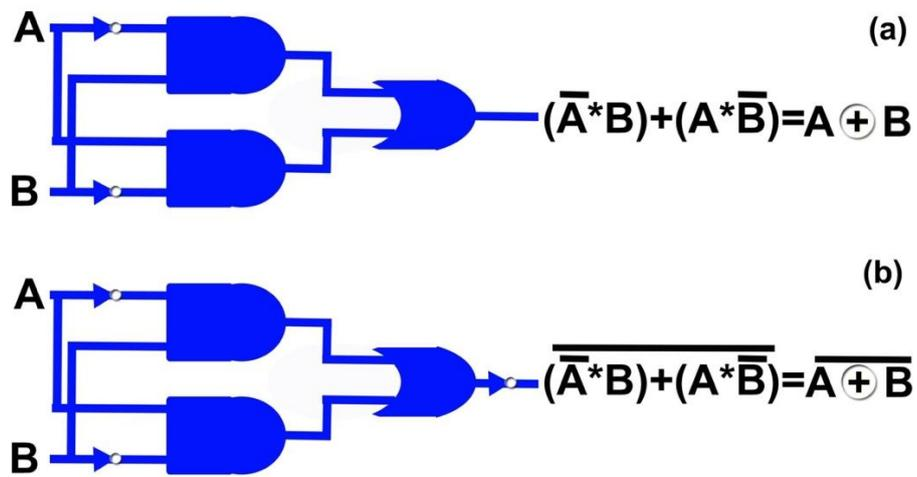
Figure 7.12 Implementation of (a) XOR and (b) NXOR by concatenation of fundamental logic gates – AND, OR and NOT
