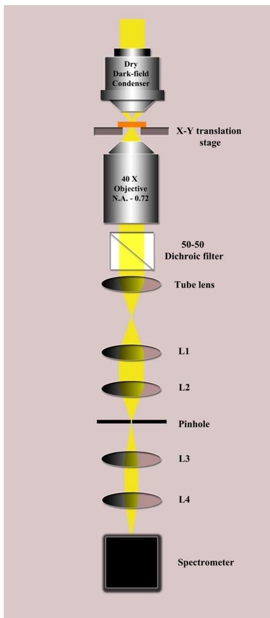
Figure 3.4 Scheme of the dark field scattering microscopy set up used during this work. The light is focussed onto the sample from top using dark-field condenser and the scattered light is collected by a 40X objective (NA = 0.72). The DF scattered signal is then passed through a pinhole placed at the conjugate image plane and the unwanted scattered signal is cut off by the pinhole. The rest of the signal is then focussed onto a spectrometer by means of convex lenses.
