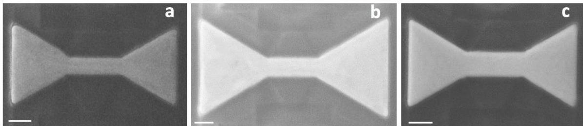
Figure 6.6 SEM images of diabolo milled with Raith Elphy multibeam pattern generator. The scale bars are 200nm.
