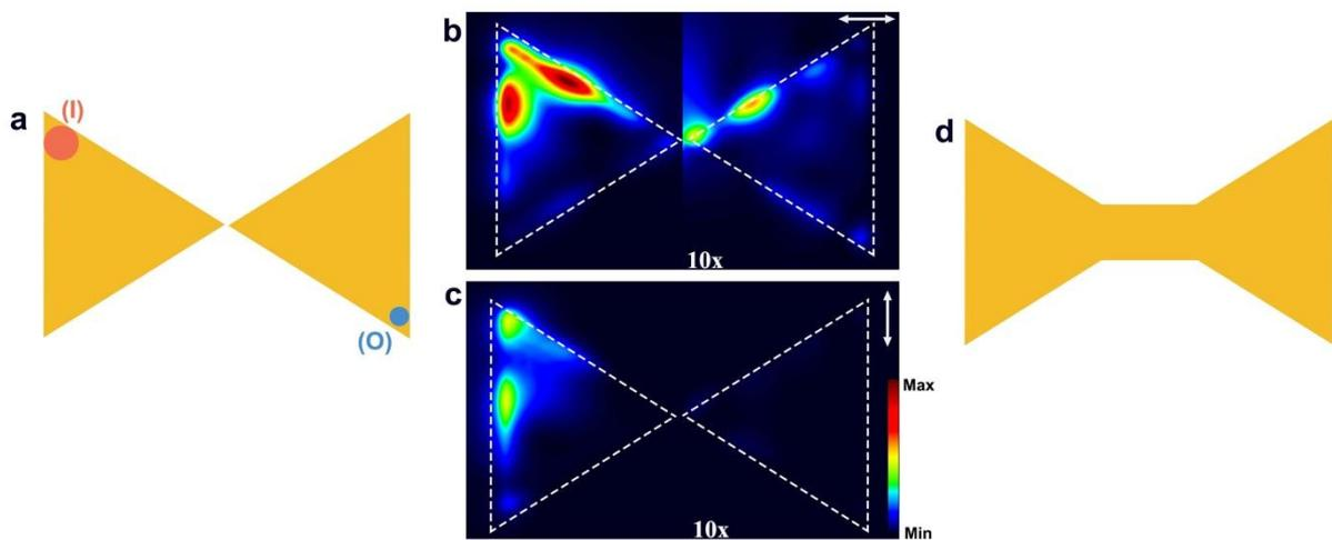
Figure 6.1 (a) Design of multimodal bowtie antennas, (b,c) Transmission image computed on a bowtie antenna with triangular prism of lateral size 925nm each for  $0^\circ$  and  $90^\circ$  in-plane polarizations respectively, (d) model of the proposed diabolo structure. The red circle on the upper left corner in (a) denotes the position of excitation and blue circle on the lower right corner denotes the output.
