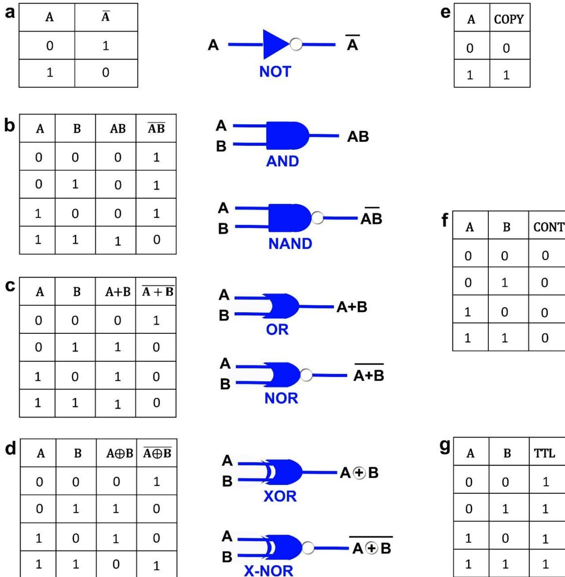
Figure 7.1 Truth table and symbols of (a) NOT gate, (b) AND and NAND gates (c) OR and NOR gates (d) XOR and X-NOR gates. Truth table of (e) Copy , (f) Contradiction and (g) Tautology respectively.
