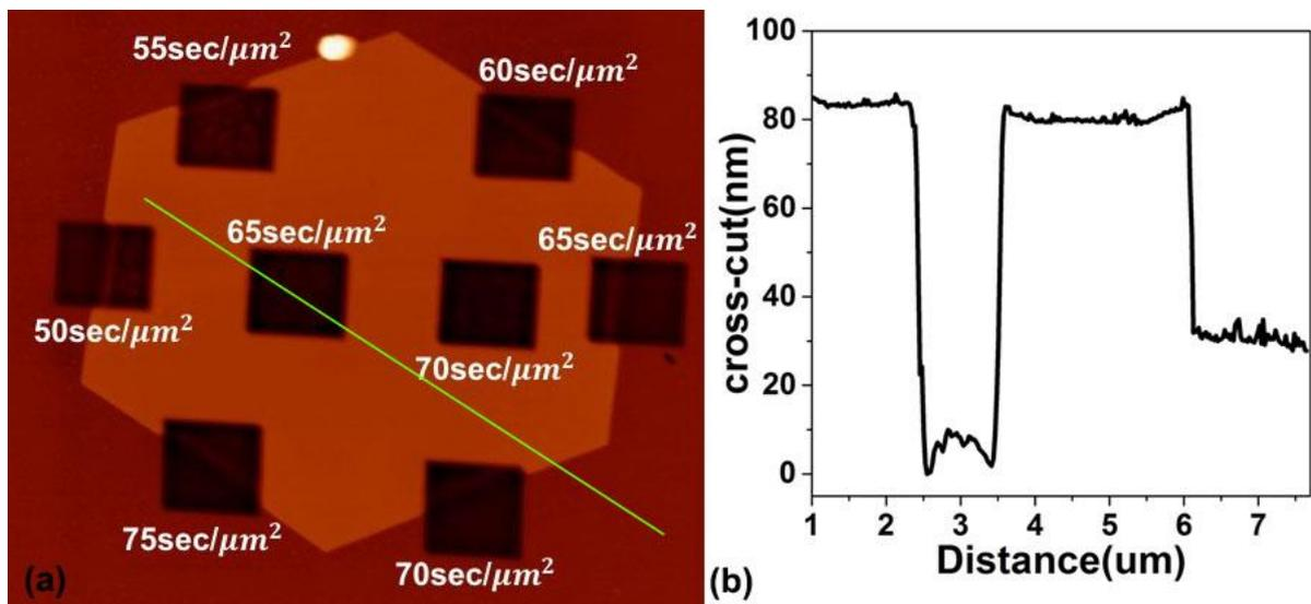
Figure 3.3 (a) AFM image of squares milled on a hexagonal gold nanoprism with milling time of 50, 55, 60, 65, 70 and 75  $\text{sec}/\mu\text{m}^2$ . The green line represents the cross-cut done on the milled hexagonal nanoprism, (b) The cross-cut profile corresponding to the green line in (a).
