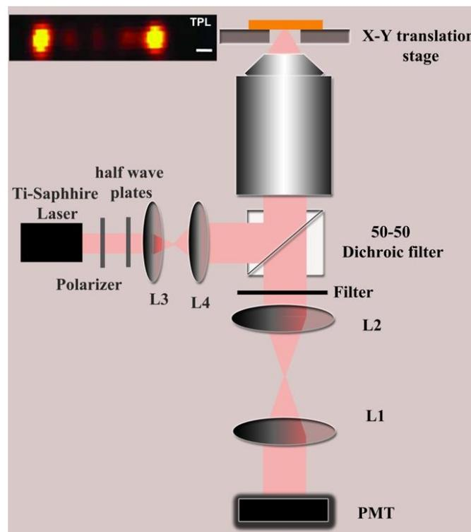
Figure 3.7 Schematic of the TPL setup used for the experimentation. Inset – Confocal TPL map of a 1500nm long nanowire. (Scale bar =200nm)
