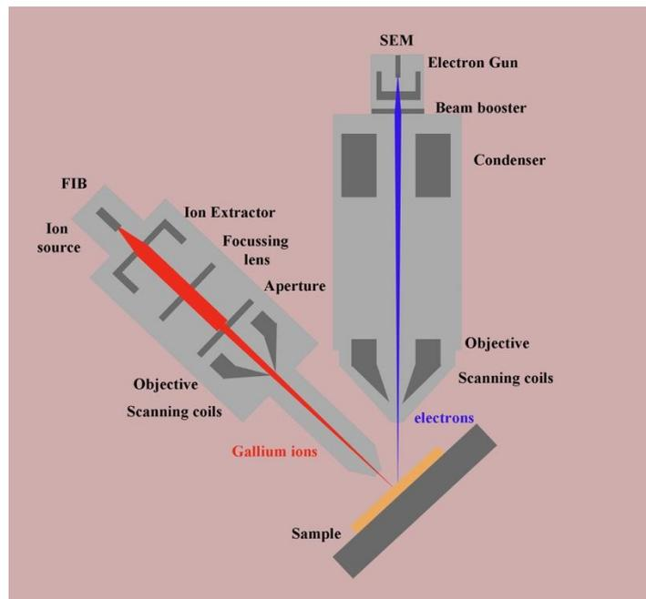
Figure 3.2 Scheme of the FIB-SEM column used for the experiments. The angle between FIB column and SEM column is 54°. The system can be used for in-situ imaging of the sample while milling is being performed.
