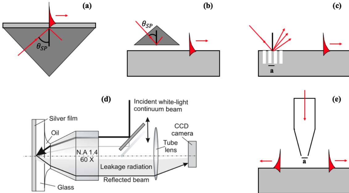
Figure 2.3 SPP excitation by means of (a, b) prism coupling in Kretschmann configuration and Otto configuration respectively, (c) grating coupling, (d) high aperture oil immersion objective lens coupling [Reprinted with permission from reference [20]] and (e) optical fibre based coupling in scanning near field microscope (SNOM).
