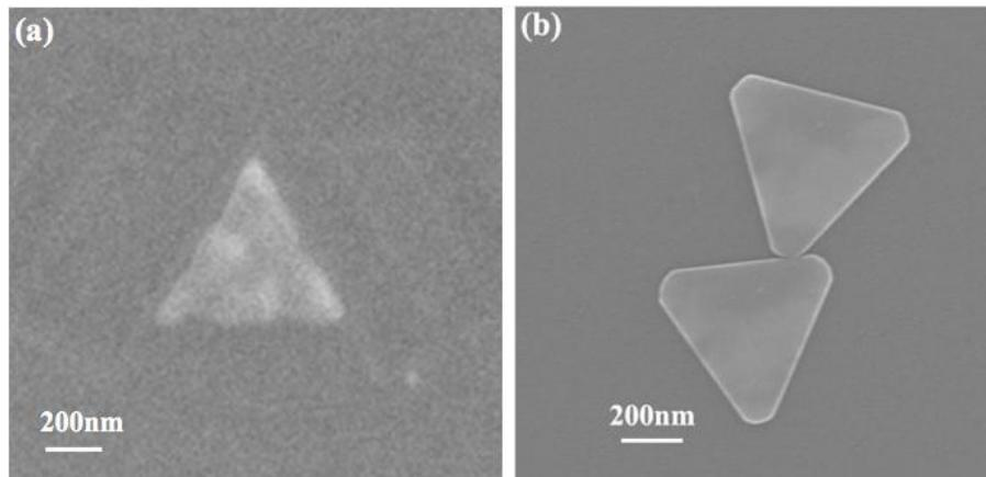
Figure 2.9 (a)SEM image of silver nanoprism obtained by focussed ion beam milling [41] of 30nm thin Ag film deposited by electron beam physical vapour deposition technique, (b) SEM image of gold nanoprism fabricated by colloidal chemistry
