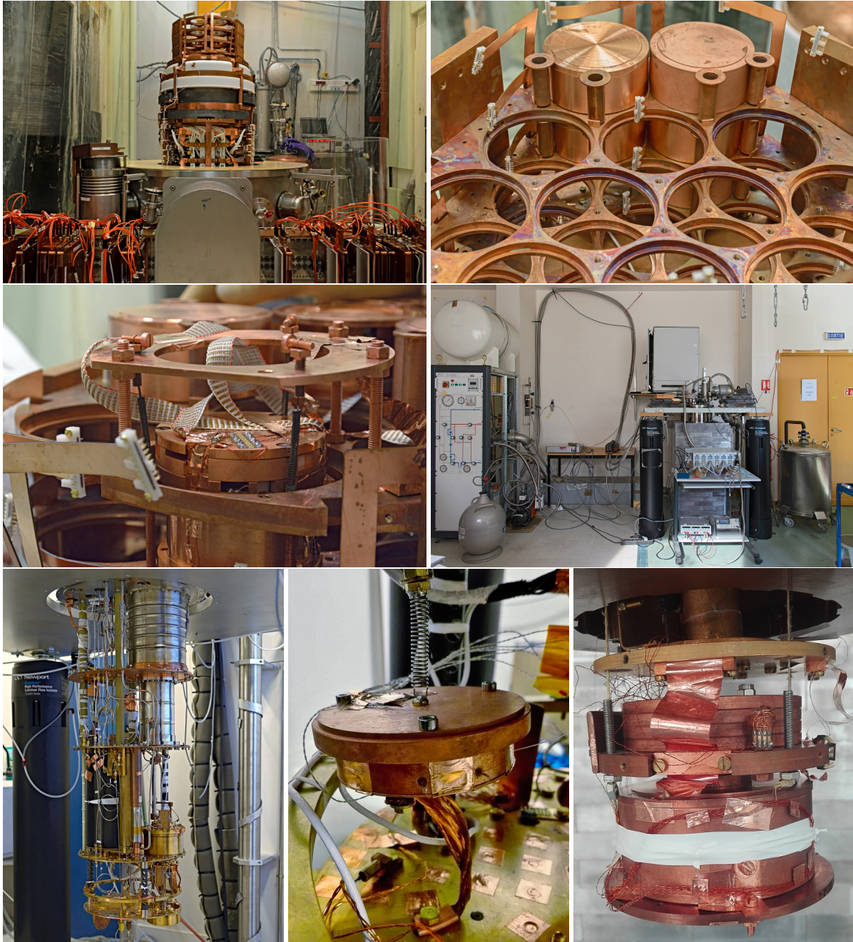
Fig. 3.5: Top-left panel: photograph of the EDELWEISS cryostat, the electronics is visible in the bottom part and the cryostat in the upper one. Top-right panel: photograph of the cryostat upper part with the galette system used to host the detectors. Galette is an internal nickname used by the EDELWEISS collaboration to refer to a set of round copper plates used to hold the detectors. As it is visible by some EDELWEISS detectors mounted, this system does not have bolometer suspension. Center-left panel: photograph of the decoupling system mounted in the EDELWEISS set-up. It is constituted by three springs to reduce the vibration effects. Center-right panel: the Ulisse cryostat test facility. Bottom-left panel: the CRYOFREE dilution unit. Bottom-middle-and-right panel: detectors mounted on the CRYOFREE and Ulisse cryostats with a spring decoupling system.
