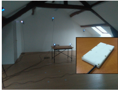
Figure 6.2: Picture of the optitrack setup. The sensor board package is displayed in the insert.
