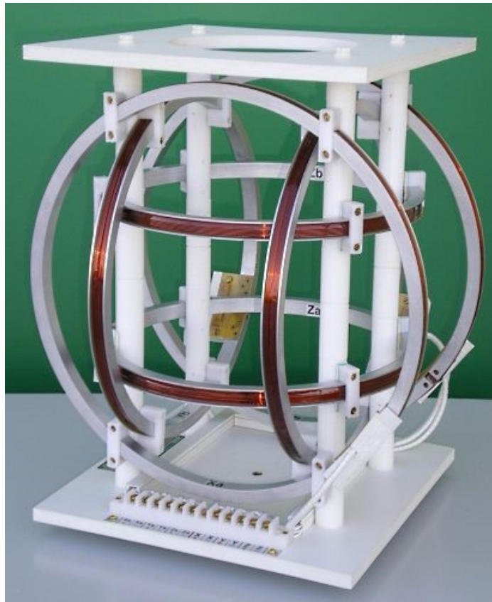
Figure 5.1: Tri-axis Ferronato® BH-600 Helmholtz coils used for this work
